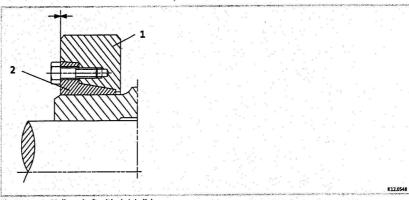
Fig. 5 Hollow shaft with shrink disk
