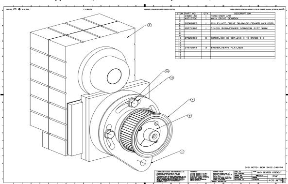
**Note:** Customers must take responsibility to ensure that the motor and gearbox pulley sets are identical across the machine.
